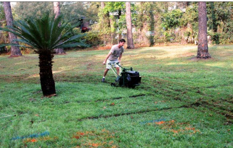
FIGURE 8.1: Walk-behind sod cutters are effective tools and often available for rent locally.
