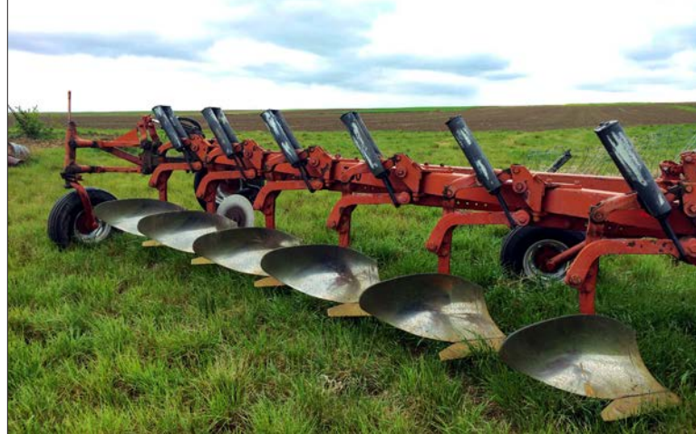
Figure 6.2: Soil inversion is ideal for flat sites that are dominated by sod-forming grasses.
