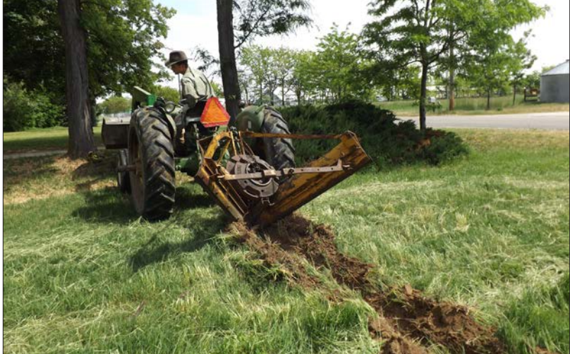
FIGURE 2.2: Walk-behind trenchers (left)—available at most equipment rental outfits—do picture-perfect trenching and can be used to prepare smaller sites that may be inaccessible to larger equipment. A variety of tractor implements can be used for trenching larger sites (right).
